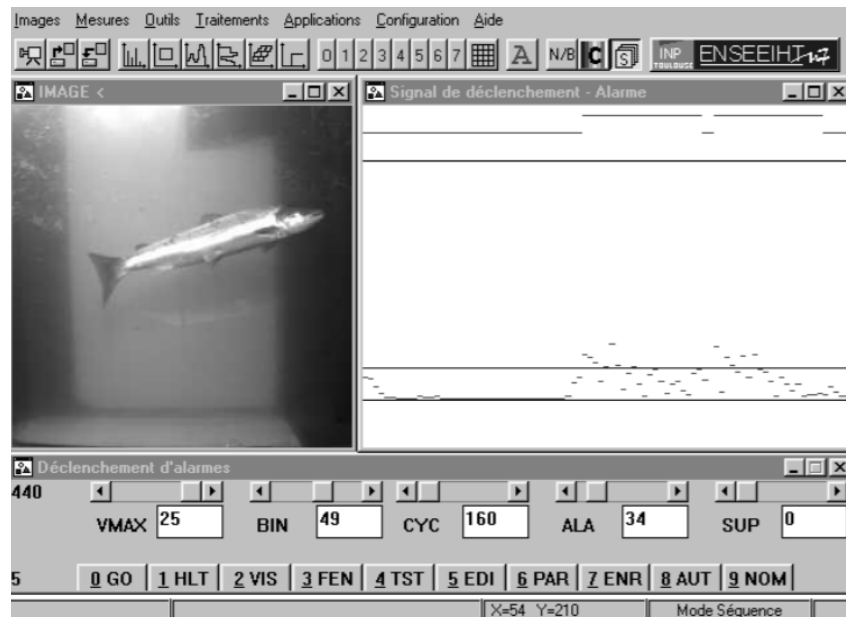
Figure 4-2. Screen image from a motion-activated fishway monitoring system
